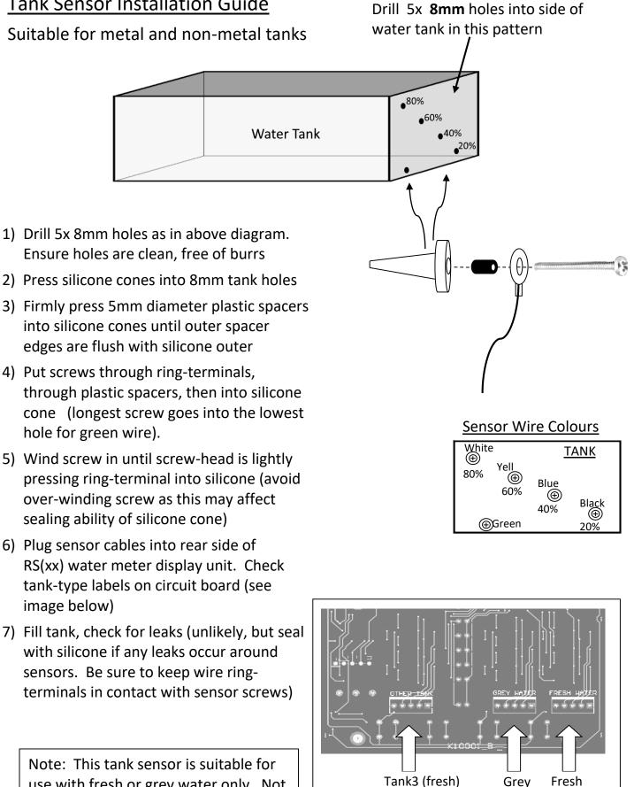
use with fresh or grey water only. Not<br/>to be used with fuel or any other<br/>liquidsTank3 (fresh)GreyFreshPlug sensor cables into rear of RS(xx) unit
